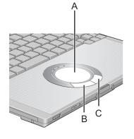
Use the touch pad to move the cursor on the screen and perform computer operations. A. Work Surface (touch pad) B. Left Button C. Right Button
